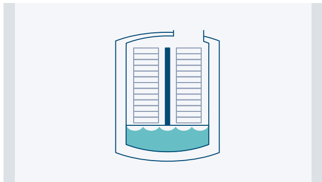
Figure 2. Vapor storage with perforated base supporting samples above LN2.
