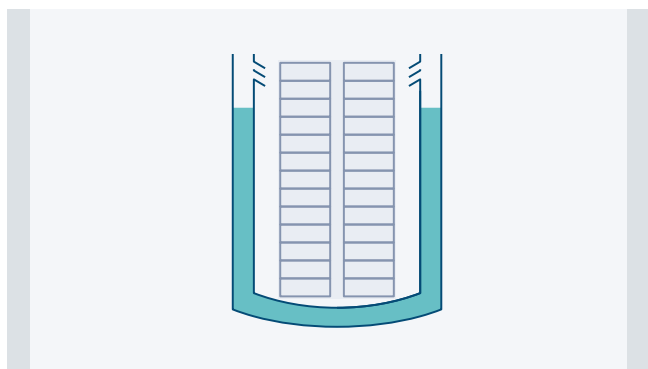
Figure 3. Isothermal freezer jacketed LN2 design providing true vapor storage.
