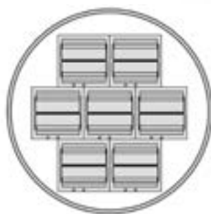
V-1500AB Square Rack configuration with capacity of 9,100 (2 mL) vials
